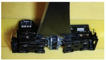
above the brass power pickup strip that was hidden behind the tank halves and gently pry until the shell lifts up a tiny bit then flip it over and do the same to the other side repeating again and again and again and again and again and again prying the shell up little by little until it pulls free. Trying to pry it out all at once or prying it up crooked, IE one side or end more than the other, will result in a broken shell.
